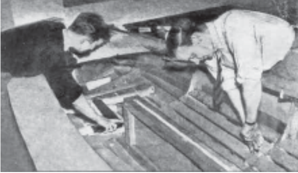
Two Pupils at work (David McLintock on the right) fixing boards inside the hull
